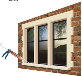
The tube contains both part A and Part B of the resin in separate compartments
